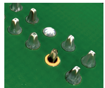
Insufficient wetting (front) and missing pin (back)
