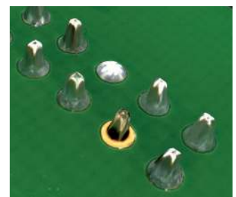
Insufficient wetting (front) and missing pin (back)
